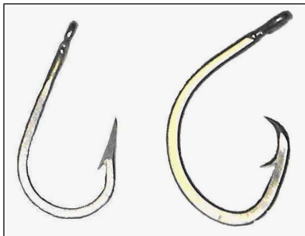
Fig. 1. 9/0 J hook manufactured by Mustad (left) 4.0 cm narrowest width, and 10 degree offset 18/0 circle hook manufactured by Lingren-Pitman 4.9 cm narrowest width (photo E. Gilman). Hooks are oriented so that the narrowest width is horizontal. Differences in hook designs other than narrowest width (i.e. orientation of point, length, gape, bite) and materials may also be important variables affecting sea turtle capture rates and position of hooking.
