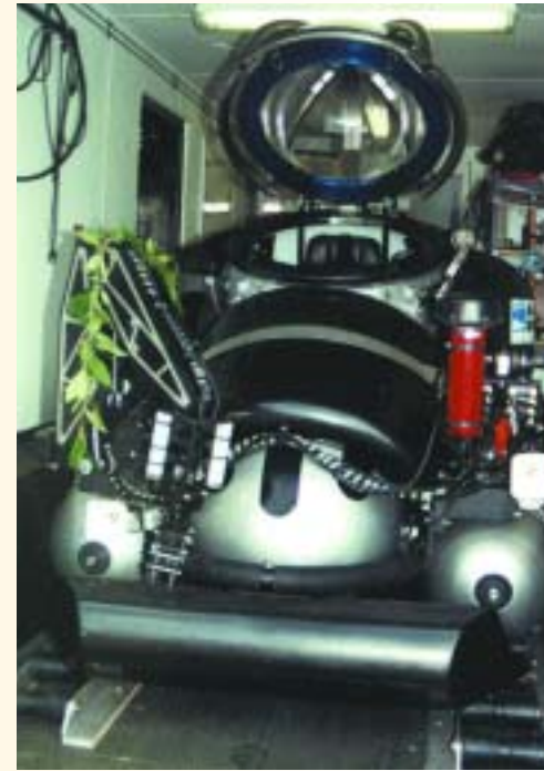
The DeepWorker—a one-person, tetherless submersible capable of working in depths down to 2,000 feet and providing a 180° field of vision—will be used to study coral reefs and determine the impacts of fisheries on them in the Hawaiian archipelago.
