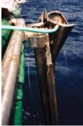
PROTECTING SEABIRDS: The underwater setting chute delivers baited hooks from the vessel so that they first emerge 16 feet underwater, out of sight and reach of diving albatrosses.
