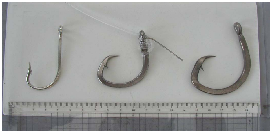
Figure 20. Hooks used in the experiment: J hook, 13/0 circle hook with wire, and 16/0 circle hook.
