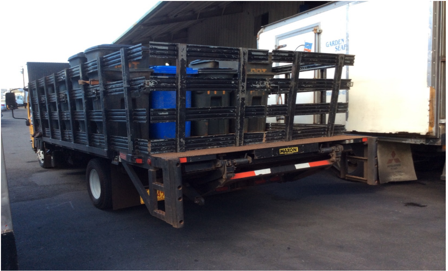
Figure 12. FPW transport for disposal. Deterioration of the fish processing waste starts when the cold chain is broken, when transported by an open uninsulated or by a non-refrigeration truck (shown above). FPW is now in ambient air temperature when it leaves the fish processor's cold room and is transported for disposal. To mitigate this deterioration process, FPW containers can be packed with ice supplied by the fish wholesaler to keep the FPW cold during transport prior to processing and would help maintain FPW quality for finished feed ingredients (fishmeal, fish silage, fish oil, fish solubles, or a ground raw frozen fish blocks). For fertilizer products from FPW, a cold chain is not required for an acceptable finished product.
