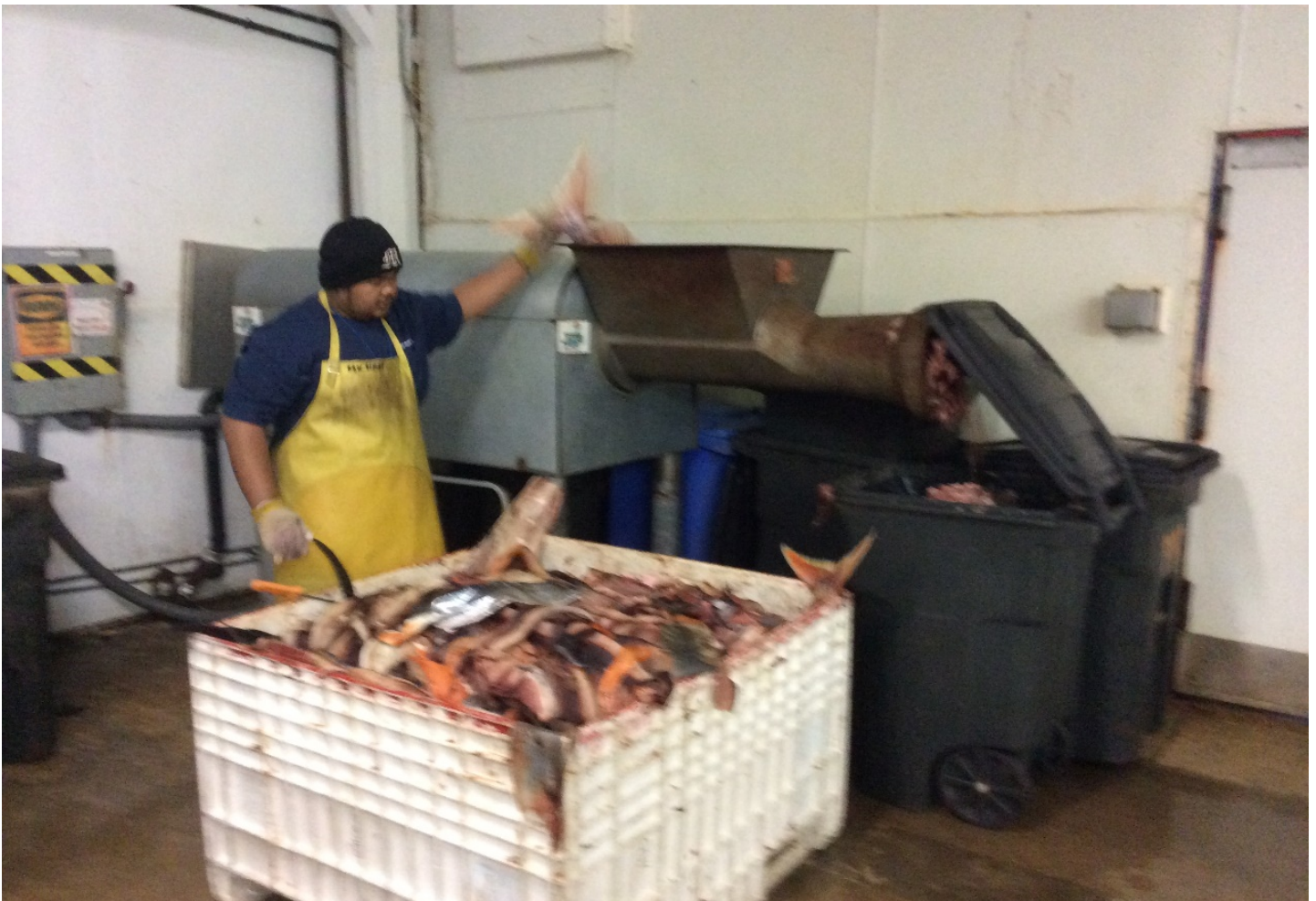
Figure 8. AUTIO GH (Gear Head) Grinder. Model 1101 GH, 1" holes die plate, notched feeder screw, weighs 2,400 lbs., with a 50 HP motor, max grinding capacity 25,000 lbs. / hr. The cost of a grinder like the Autio model 1101 GH is about $36,500, a soft start is needed for the 50 HP motor which costs about $4,000, add shipping and handling about $2,000. Total cost of Grinder is approximately $42,600 + the cost of installation.
