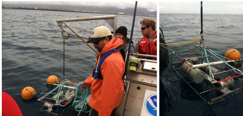
MOUSS system setup and deployment were field-tested during March and April 2015 using a 19-foot NOAA Safe Boat.
