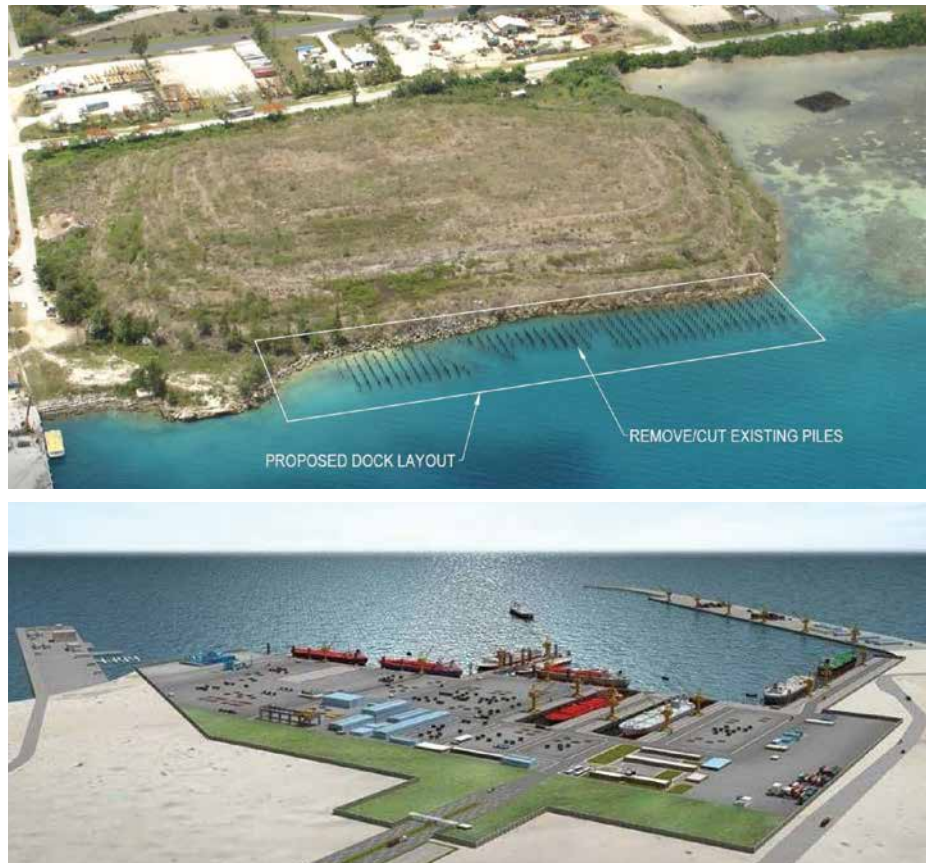
Top: Aerial photo of Puerto Rico Dump showing the proposed dock layout and existing I-beam steel piles. Above: Artist's rendering of dock with support facilities.
