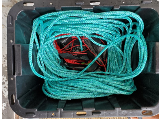
Figure 12. 105 m short streamer line being shown here coiled into a black plastic 12-gal bin. Captains like that the bin was small, portable, and easily stored away on vessels with limited deck space.
