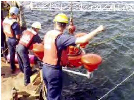
The USCG uses special skimmers to contain and recapture fuel spills. Photo: Gary Chalker/USCG
