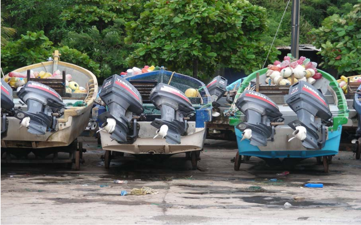
Fig.6 Longline fishing vessels made of fiberglass with an outboard motor
