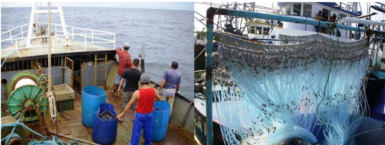
Fig. 3a and 3b: Hydraulic reel for mainline and storage bins for branchlines 3a (left), and hanger ropes for branchlines 3b (right)
