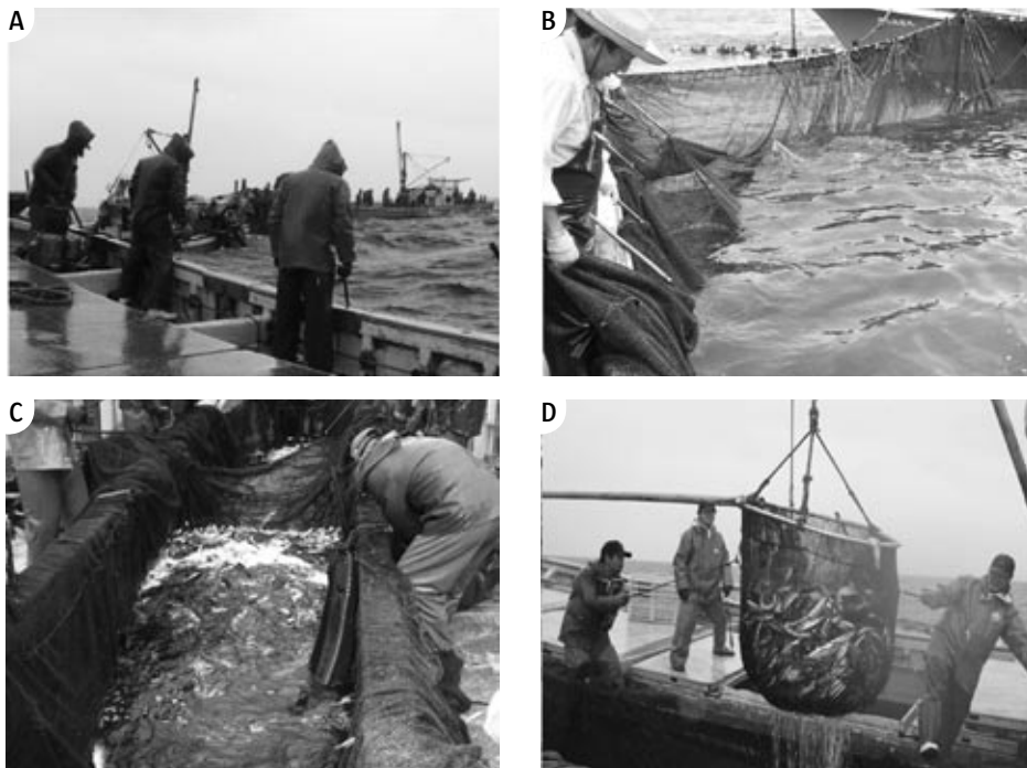
FIGURE 3. The process of collecting fish out of a pond net (A to D).
