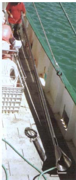
The underwater setting chute stored on deck. The chute is 27 feet long. When deployed 16 feet is underwater. © E. Gillman
