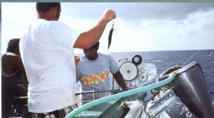
The underwater setting chute delivers baited hooks from the vessel so that they first emerge 16 feet underwater, out of sight and reach of diving albatross. © E. Gillman
