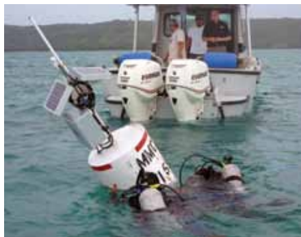
Fred Hegg (in black shirt) of Falmouth Engineering was on Saipan the week of Aug. 2, 2010, to help the CNMI Division of Fish and Wildlife (DFW) to install telemetric sensors on five buoys. Pictured is the first buoy, deployed for testing purposes. Within minutes, data on water salinity, temperature and current were being captured and transmitted to a laptop onboard the DFW vessel. The buoys will be deployed in September, three inside Saipan lagoon and two about 7 miles west of Saipan. The project is funded by the Western Pacific Regional Fishery Management Council through a grant from the NOAA Coral Reef Conservation Program.
