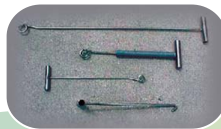
Four types of dehooking devices that can be used to safely release hooked sea turtles. By removing hooks and releasing turtles, chances of survival are increased and post-hooking mortality is reduced.
