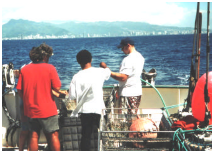
Figure 5. When setting, the mainline is set through a line setting machine (to the left), baited hooks are sent through the underwater setting chute (to the right of the crew), and the branch line with the baited hook is clipped onto the mainline moments after the baited hook is sent through the chute.
