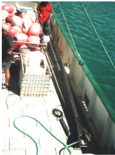
Figure 4. The underwater setting chute is stored on deck against the bulwarks. The chute is 9 meters long, and when deployed, 5.4 meters of the chute's shaft is underwater.
