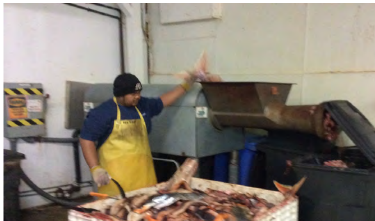
Figure 8 Autio GH (Gear Head) Grinder. Model 1101 GH, 1" holes die plate, notched feeder screw, weighs 2,400 lbs., with a 50 HP motor, max grinding capacity 25,000 lbs. per hour. The cost of a grinder like the Autio model 1101 GH is about $36,500. A soft start is needed for the 50 HP motor, which costs about $4,000, add shipping and handling about $2,000. Total cost of grinder is approximately $42,600 plus the cost of installation.
