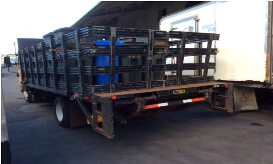
Figure 12 FPW transport for disposal. Deterioration of the FPW starts when the cold chain is broken, when transported by an open uninsulated or by a non-refrigeration truck (shown above). FPW is now in ambient air temperature when it leaves the fish processor's cold room and is transported for disposal. To mitigate this deterioration process, FPW containers can be packed with ice supplied by the fish wholesaler to keep the FPW cold during transport prior to processing. and would help maintain FPW quality for finished feed ingredients (fishmeal, fish silage, fish oil, fish solubles, or a ground raw frozen fish blocks). For fertilizer products from FPW, a cold chain is not required for an acceptable finished product.
