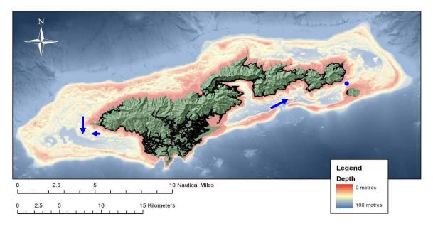
Figure 18. Summary residual flow. Good data so far is only available from the channel between Aunu'u and the mainland, Taema bank and the western tip of the island.
