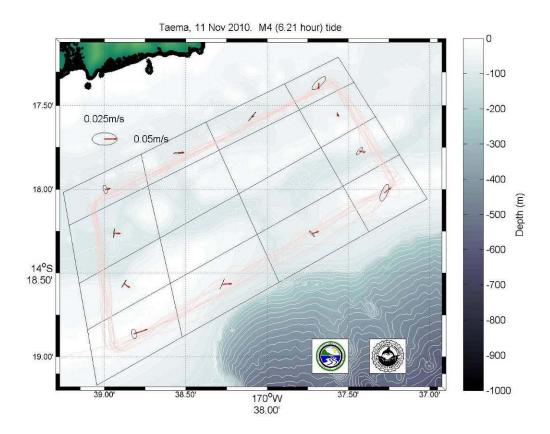
Figure 9. M4 tidal component around Taema bank.
