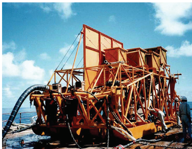
Manganese nodule collector. Photo courtesy COMRA.
