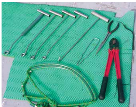
Examples of sea turtle safe handling gear required for Hawai'i-based longline vessels. These gear help remove hooks and other gear from sea turtles before release.
