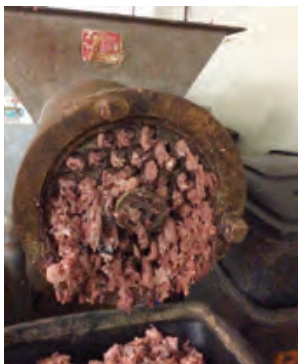
An SK-funded project in the Western Pacific Region researched conversion of fish waste into fish silage. Pictured is a grinder to macerate the fish discards.
