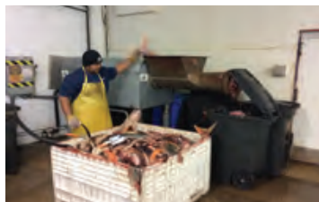
An SK-funded project in the Western Pacific Region researched conversion of fish waste into fish silage. Pictured is a grinder to macerate the fish discards.
