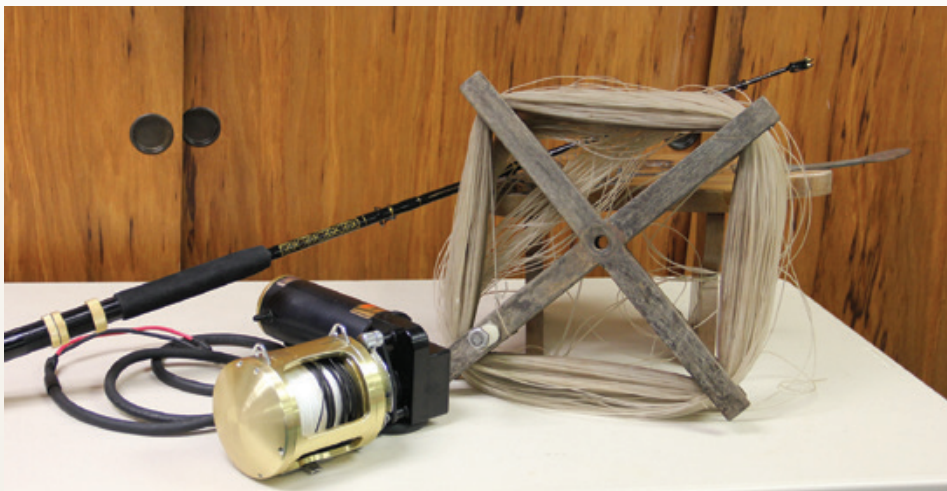
For decades, traditional wooden hand-cranked reels have been used by American Samoa bottomfish fishermen, including most alia fishermen, since modern fiberglass rods and electric reels are expensive and not readily available.
