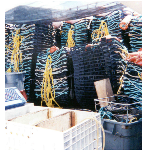
Fig. 14. The plastic traps opened quickly into identical halves for easy stacking, allowing many traps to be stored on deck. Photo: NOAA.
