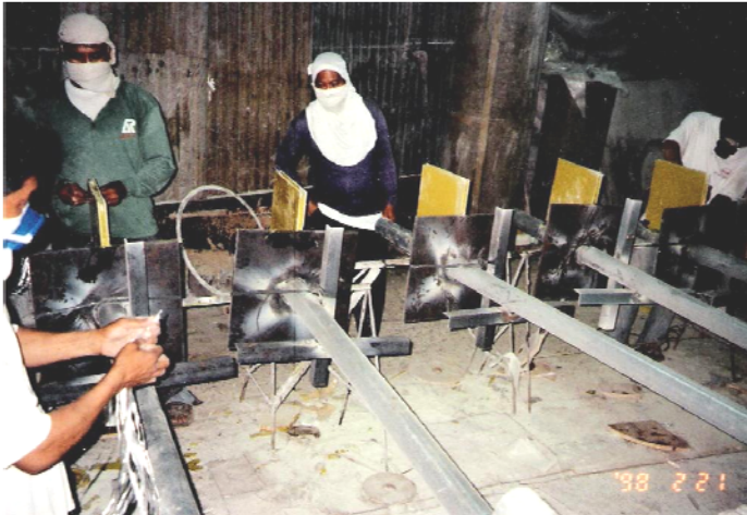
Figure 3: Internal buoy structure with 9 foot, 3 inch diameter pipe and two angle bars for support. The yellow panel is the keel (
