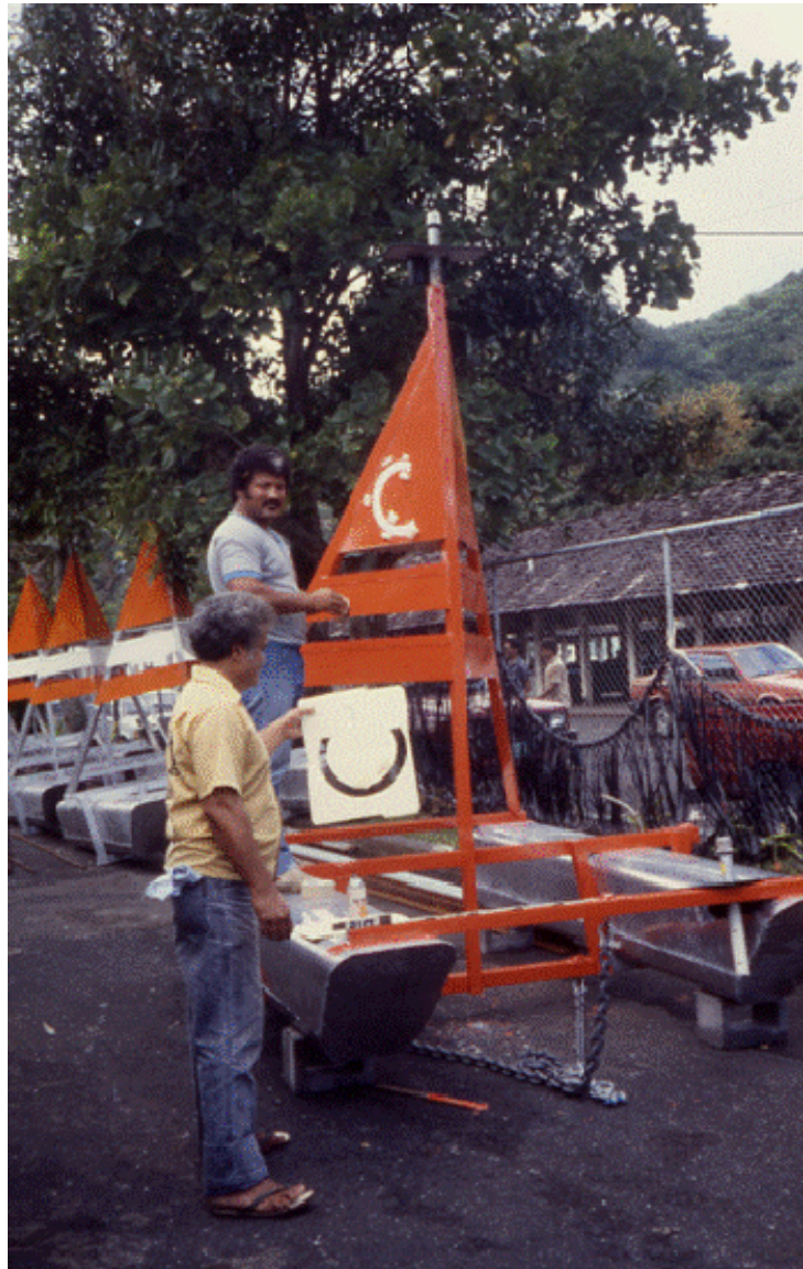
Figure 15. Catamaran style FAD float in American Samoa, c. 1986. Note polypropylene strapping appendages buckled to chain links.
