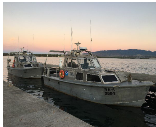
Figure 11. Rainier is equipped with two highly sophisticated hydrographic launches and two dive boats that will all be deployed daily to conduct NCRMP surveys and mapping in the region.
