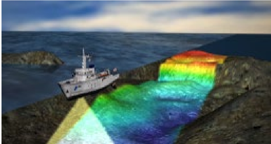
Figure 9. Graphic of a NOAA survey vessel scanning the ocean floor using multibeam sonar.
