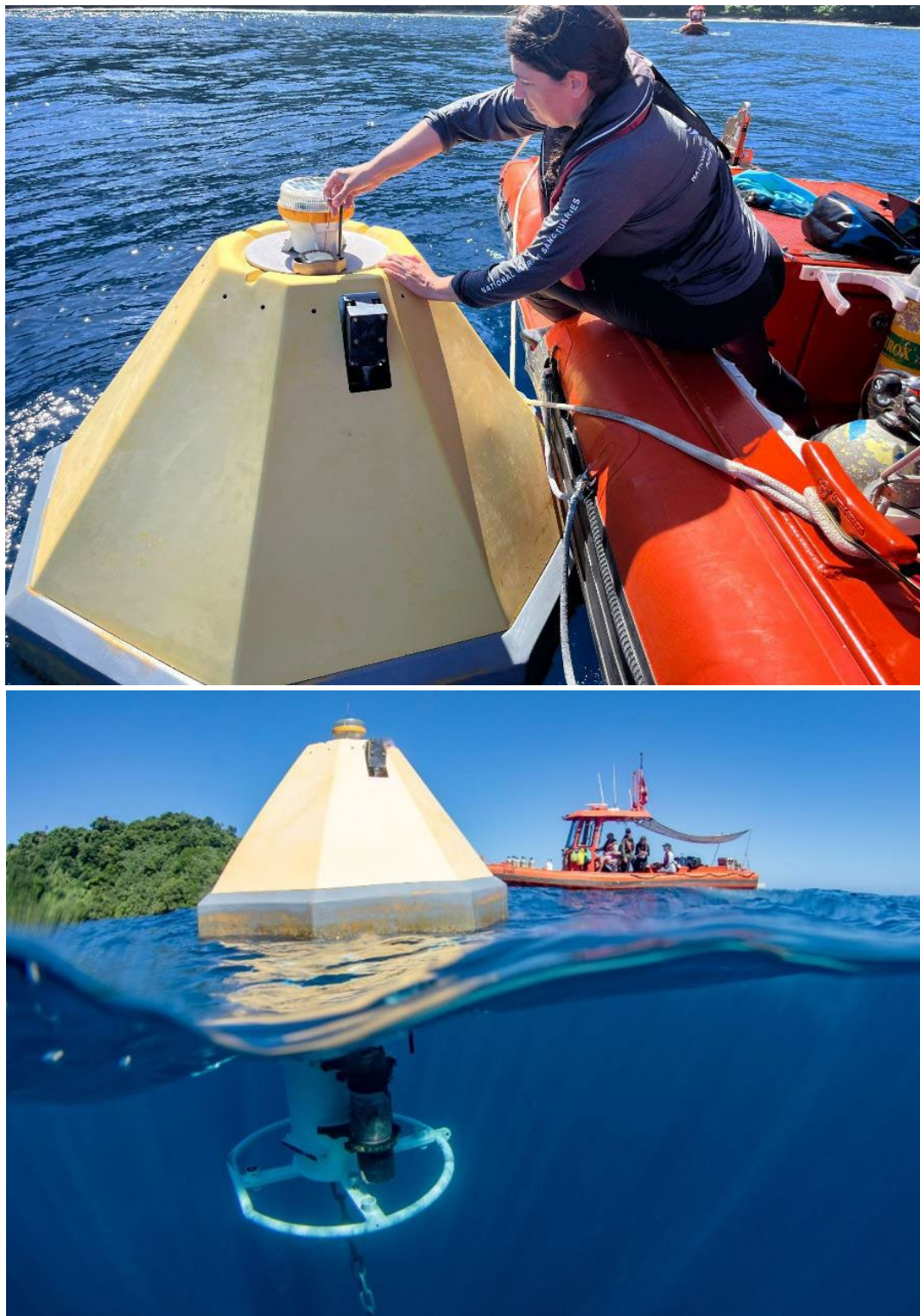
The OCC Team assisted NOAA Sanctuaries scientist Valerie Brown while she programmed the oceanographic instruments in the CO 2 buoy that monitors ocean acidification in Fagatele Bay. Photo credits: NOAA Fisheries. Photographers: Joy Smith (top); Jeff Milisen (bottom).
