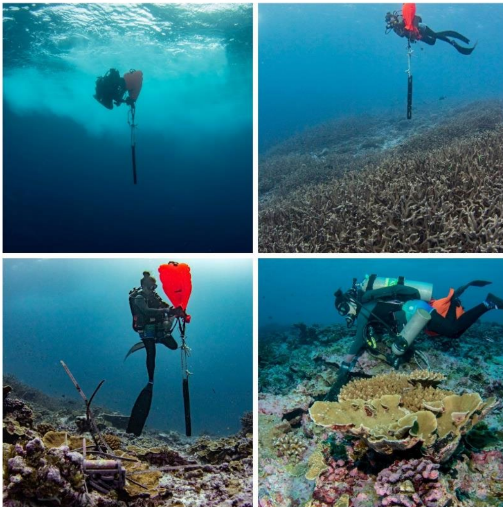
A diver uses a bag filled with air to help deploy an acoustic recorder. Photo credit: NOAA Fisheries. Photographer: Jeff Milisen.
