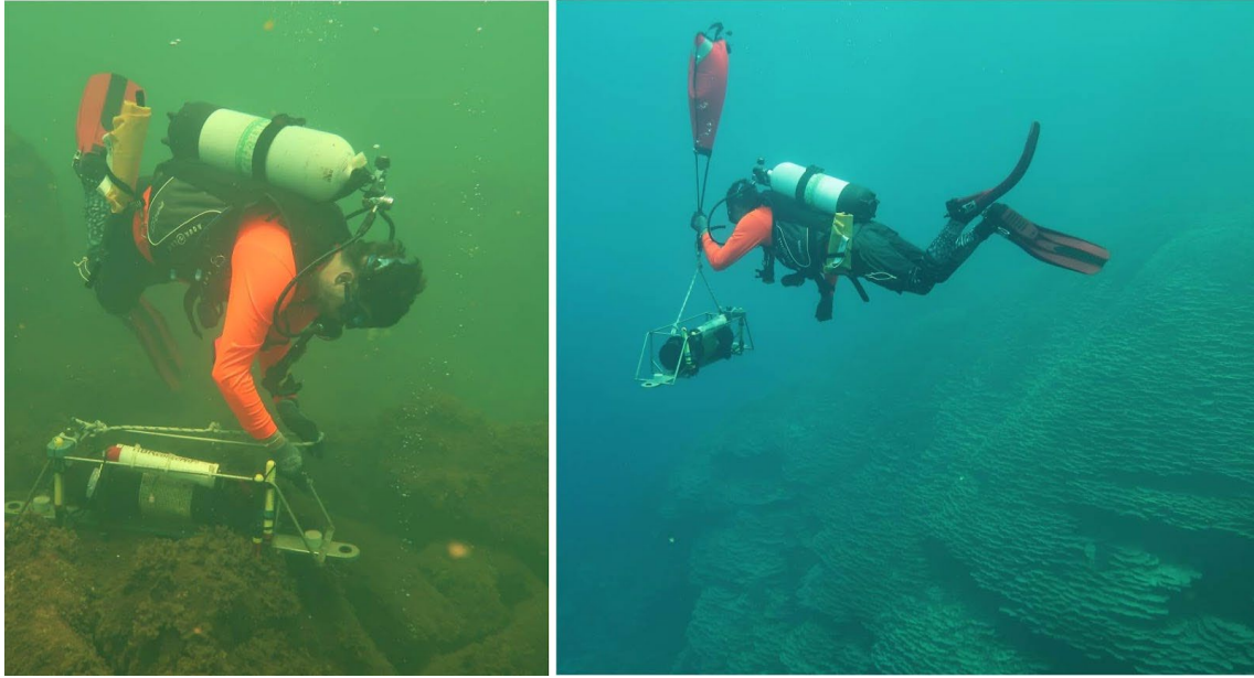
Scientists at Maug caldera use lift bags filled with air to help move heavy instruments carefully down to the seafloor. Credit: NOAA Fisheries / Zach Taylor
